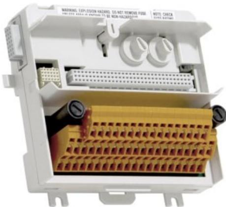
The TU833 MTU can have up to 16 I/O channels and two process voltage connections. Each channel has two I/O connections and one ZP connection. The process voltage can be connected to two individually isolated groups. Each group has a 6.3 A fuse. The maximum rated voltage is 50 V and maximum rated current is 2 A per channel. It is recommended that the fuse rating be chosen to meet the applications needs, see S800 I/O Getting Started chapter Power and Cooling.
