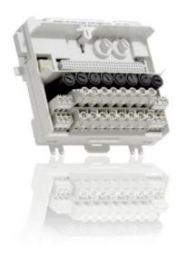
The TU837V1 MTU can have up to 8 I/O channels. The maximum rated voltage is 250 V and maximum rated current is 3 A per channel. The MTU distributes the ModuleBus to the I/O module and to the next MTU. It also generates the correct address to the I/O module by shifting the outgoing position signals to the next MTU.
