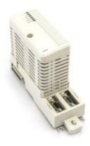
PROFIBUS DP is a high speed multipurpose bus protocol (up to 12Mbit/s) for interconnecting field devices, like remote I/O, drives, low voltage electrical equipment, and controllers. PROFIBUS DP can be connected to the AC 800M via the Cl854B communication interface. The Cl854B includes two PROFIBUS ports to realize line redundancy and it also supports PROFIBUS master redundancy.
