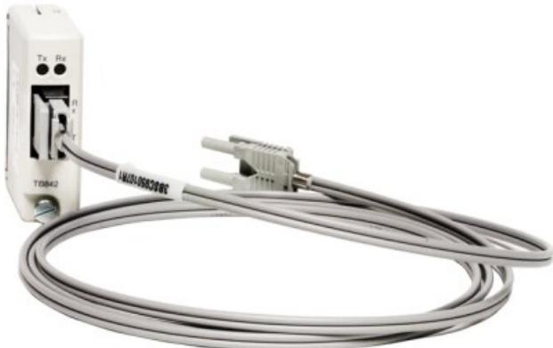
TB842 ModuleBus Optical Port is a communication interface between the CI801 or CI840/CI840A FCI and the TB820/TB820V2/TB840/TB840A ModuleBus modem of an I/O cluster or ABB drives units via the Optical ModuleBus. TB842 connects to CI801 via TB806 and to CI840/CI840A via TU847 and TB806 for single I/O or via TU846 and TB846 for redundant I/O.
