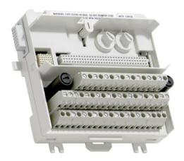
The TU839 MTU can have up to 8 I/O channels and two groups of connections for sensor power distribution. Each channel has two I/O connections. The process voltage can be connected to two individually isolated groups for sensor power distribution. Each group has a 200 mA fuse. The maximum rated voltage is 250 V and maximum rated current is 1 A per channel. It is recommended that the fuse rating be chosen to meet the applications needs.
