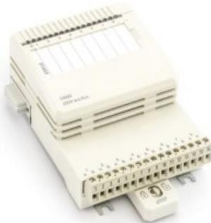
The DI803 is an 8 channel 230 V a.c./d.c. digital input module for the S800 I/O. This module has 8 digital inputs. The a.c. input voltage range is 164 - 264 volt and the input current is 7.6 mA at 230 V a.c. The d.c. input range is 175 - 275 V and the input current is 1.6 mA at 220 V. The inputs are individually isolated. Every input channel consists of current limiting components, EMC protection components, input state indication LED and optical isolation barrier.
