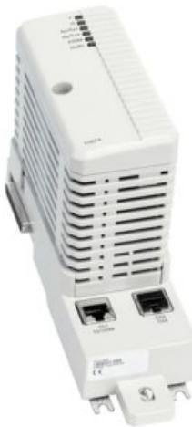
The CI874 is an AC 800M communication interface that connects to external Ethernet devices using the OPC UA protocol. The TP867 Baseplate has one RJ45 Ethernet connector that supports 100Mbps. The CI874 expansion unit contains the CEX-Bus logic, a communication unit, and a DC/DC converter that supplies the required voltage from +24 V supply through the CEX-Bus.
