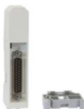
The TB806 ModuleBus Cable Adaptor is used together with TB805 and TK801V0xx to extend the ModuleBus. Using this extension I/O modules on the same electrical ModuleBus can be mounted on different DIN rails. TB806 can also be used together with TB842 to provide an optical extension of the ModuleBus.
