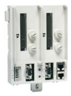
The TU847 is a module termination unit (MTU) for redundant configuration of the field communication interface Cl840/Cl840A. The MTU is a passive unit having connections for power supply, electrical ModuleBus, two Cl840/Cl840A and two rotary switches for station address (0 to 99) settings. A ModuleBus Optical Port TB842 can be connected to TU847 via TB806.
