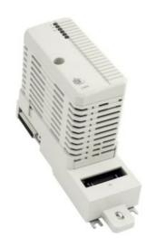
S100 I/O communication is realized in AC 800M by communication interface CI856, which is connected to the CEX-Bus through a base plate. The baseplate, TP856, houses a ribbon connector connecting to bus extender boards in S100 I/O racks and provides a simple DIN-rail mounting. Up to five S100 I/O racks can be connected to one CI856 where each I/O rack can hold up to 20 I/O boards.
