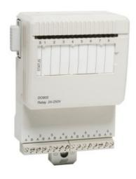
The DO802 is an 8 channel 110 V d.c./250 V a.c. relay (NO) output module for the S800 I/O. The maximum voltage range is 250 V and the maximum continuous output current is 2 A. All outputs are individually isolated. Each output channel consists of optical isolation barrier, output state indication LED, relay driver, relay and EMC protection components.
