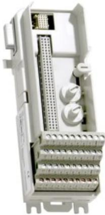
The TU818 is a 32 channel 50 V compact module termination unit (MTU) for the S800 I/O. The MTU is a passive unit used for connection of the field wiring to the I/O modules. It also contains a part of the ModuleBus.
