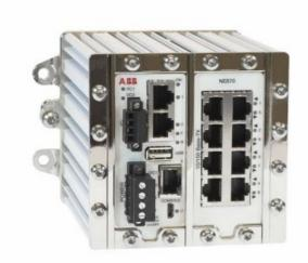
NE870 is an industrial router that also acts as a firewall. The router/firewall can be utilized to segment a system into network areas and also security zones. NE870 is primarily intended to be used to separate client/server networks and control networks, to separate different control and safety networks, and also to create RNRP tunnel areas between RNRP networks.
