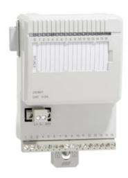
The DO801 is a 16 channel 24 V digital output module for the S800 I/O. The output voltage range is 10 to 30 volt and the maximum continuous output current is 0.5 A. The outputs are protected against short circuits, over voltage and over temperature. The outputs are in one isolated group. Each output channel consists of a short circuit and over temperature protected high side driver, EMC protection components, inductive load suppression, output state indication LED and optical isolation barrier.
