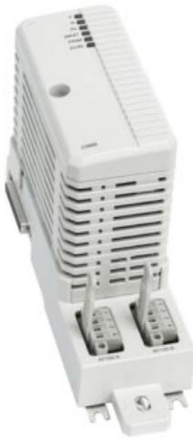
The CI869 is an AC 800M communication interface that connects to the AF 100 field bus through the twisted pair (TWP). The CI869 expansion unit contains the CEX-Bus logic, a communication unit, and a DC/DC converter that supplies the required voltage from +24 V supply through the CEX-Bus. The CI869 can be configured for both redundant cables and redundant communication interfaces.
