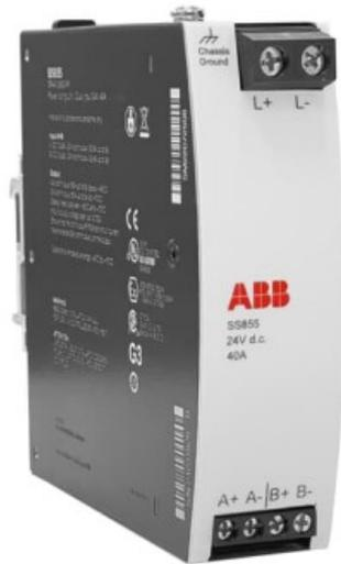
The SS855 is a voting unit for building redundant power supply systems. It is equipped with two input channels and one output. The two inputs are decoupled by MOSFET technology.
