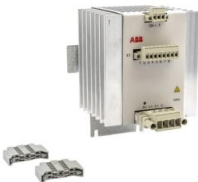
The Voting Units SS823 and SS832 have been specifically designed to work as control units within a redundant power supply configuration. The output connections from two Power Supply Units are connected to the Voting Unit.
