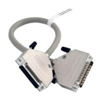
The TK801V003 ModuleBus Extension Cable is a 0.3 m long cable that is used together with TB805/TB845 and TB806/TB846 to extend the ModuleBus. Using this extension I/O modules on the same electrical ModuleBus can be mounted on different DIN rails.
