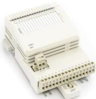
The DI801 is a 16 channel 24 V digital input module for the S800 I/O. This module has 16 digital inputs. The input voltage range is 18 to 30 volt d.c. and the input current is 6 mA at 24 V. The inputs are in one isolated group with sixteen channels and channel number sixteen can be used for voltage supervision input in the group. Every input channel consists of current limiting components, EMC protection components, input state indication LED and optical isolation barrier.
