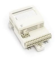
The DI801 is a 16 channel 24 V digital input module for the S800 I/O. This module has 16 digital inputs. The input voltage range is 18 to 30 volt d.c. and the input current is 6 mA at 24 V. The inputs are in one isolated group with sixteen channels and channel number sixteen can be used for voltage supervision input in the group. Every input channel consists of current limiting components, EMC protection components, input state indication LED and optical isolation barrier.
