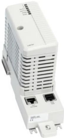
The CI873A is an AC 800M communication interface that connects to external Ethernet devices using the EtherNet/IP protocol. The TP867 Baseplate has two RJ45 Ethernet connectors, but only the CH1 connector that supports 100Mbps is used. The CI873 expansion unit contains the CEX-Bus logic, a communication unit, and a DC/DC converter that supplies the required voltage from +24 V supply through the CEX-Bus.
