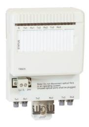
S800 I/O is a comprehensive. distributed and modular process I/O system that communicates with parent controllers and PLCs over industry-standard field buses. The TB825 ModuleBus Optical media converter, converts between plastic opto fiber or HCS fiber with versatile link connectors and glass optical fiber with ST connectors.
