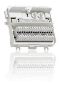
The TU851 MTU can have up to 16 I/O channels. The maximum rated voltage is 250 V and maximum rated current is 3 A per channel. The MTU distributes the ModuleBus to the I/O module and to the next MTU. It also generates the correct address to the I/O module by shifting the outgoing position signals to the next MTU.
