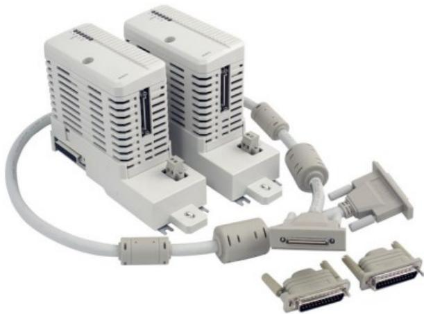
The BC810 unit consists of two basic parts: baseplate (TP857) and power supply/logic board. The baseplate is where the connectors to CEX-Bus and the external power reside. It is grounded to the DIN-rail through metal parts of the housing. The board also carries the external power voting diode and fuse. The power supply and logic board contain the +3.3 V converter, logic, drivers for CEX-Bus interconnection, and the connector for the interconnection cable.
