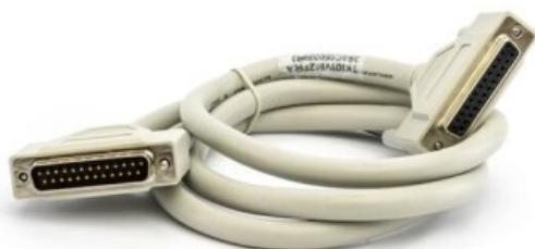
The TK801V012 ModuleBus Extension Cable is a 1.2 m long cable that is used together with TB805/TB845 and TB806/TB846 to extend the ModuleBus. Using this extension I/O modules on the same electrical ModuleBus can be mounted on different DIN rails.
