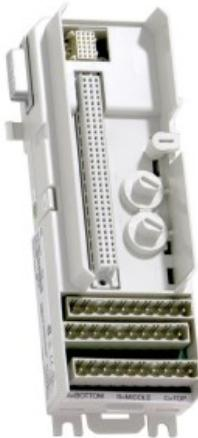
The TU814V1 MTU can have up to 16 I/O channels and two process voltage connections. The maximum rated voltage is 50 V and maximum rated current is 2 A per channel.
