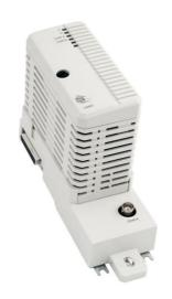
The CI865 module is the AC 800M system's communication interface for Satt ControlNet and bridges different bus standards used on AC 800M and Satt ControlNet. The CI865 module makes it possible to use older Satt I/O system (Rack I/O and Series 200 I/O) with the AC 800M controller platform, but it cannot be used as a general ControlNet interface. CI865 cannot be used in a High Integrity controller.
