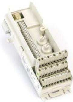
The TU811V1 is a 8 channel 250 V compact module termination unit (MTU) for the S800 I/O. The MTU is a passive unit used for connection of the field wiring to the I/O modules. It also contains a part of the ModuleBus.
