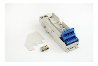
The TU891 is a compact MTU for the S800 I/O. The MTU is a passive unit used for connection of the field wiring and power supply to the I/O modules. It also contains a part of the ModuleBus. The TU891 MTU has gray terminals for field signals and process voltage connections. The maximum rated voltage is 50 V and maximum rated current is 2 A per channel, but these are primarily constrained to specific values by the design of the I/O modules for their certified application.
