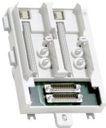
The TU852 is a 16 channel module termination unit (MTU) for redundant S800 I/O modules and for mounting on a horizontal DIN rail. The MTU is a passive unit used for connection of the field wiring to the I/O modules. It also contains a part of the ModuleBus.
