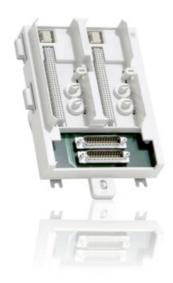
The TU852 is a 16 channel module termination unit (MTU) for redundant S800 I/O modules and for mounting on a horizontal DIN rail. The MTU is a passive unit used for connection of the field wiring to the I/O modules. It also contains a part of the ModuleBus.
