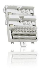
The TU845 MTU can have up to 8 I/O channels and 2+2 process voltage connections. Each channel has two I/O connections and one ZP connection. Input signals are connected via individual shunt sticks, TY801. The shunt stick is used to choose between voltage and current input. The maximum rated voltage is 50 V and maximum rated current is 2 A per channel.
