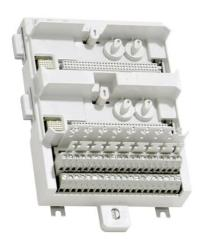
The TU845 MTU can have up to 8 I/O channels and 2+2 process voltage connections. Each channel has two I/O connections and one ZP connection. Input signals are connected via individual shunt sticks, TY801. The shunt stick is used to choose between voltage and current input. The maximum rated voltage is 50 V and maximum rated current is 2 A per channel.
