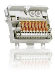
The TU836V1 MTU can have up to 8 I/O channels. The maximum rated voltage is 250 V and maximum rated current is 3 A per channel. The MTU distributes the ModuleBus to the I/O module and to the next MTU. It also generates the correct address to the I/O module by shifting the outgoing position signals to the next MTU.
