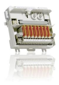
The TU835V1 MTU can have up to 8 I/O channels. The maximum rated voltage is 50V and maximum rated current is 2 A per channel. The MTU distributes the ModuleBus to the I/O module and to the next MTU. It also generates the correct address to the I/O module by shifting the outgoing position signals to the next MTU.
